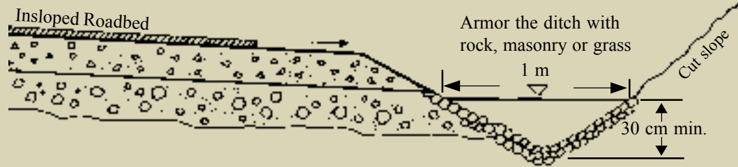
b. Typical Ditch Armoring and Shape
