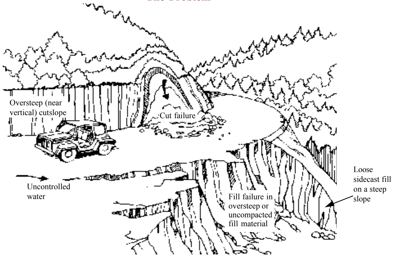
Figure 11.3 Slope problems and solutions with stabilization measures.
